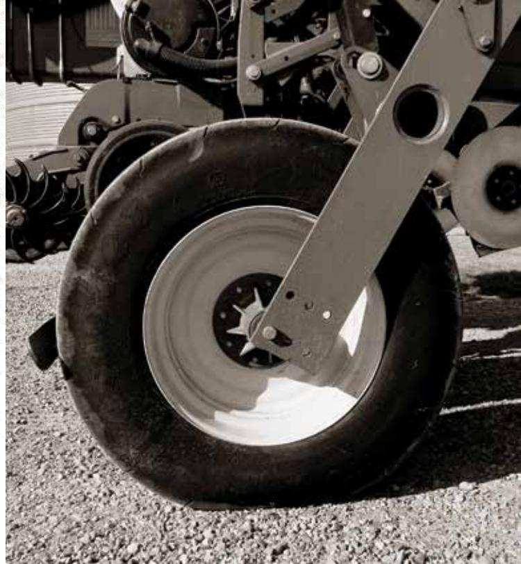
A wider section width may significantly reduce soil compaction.
