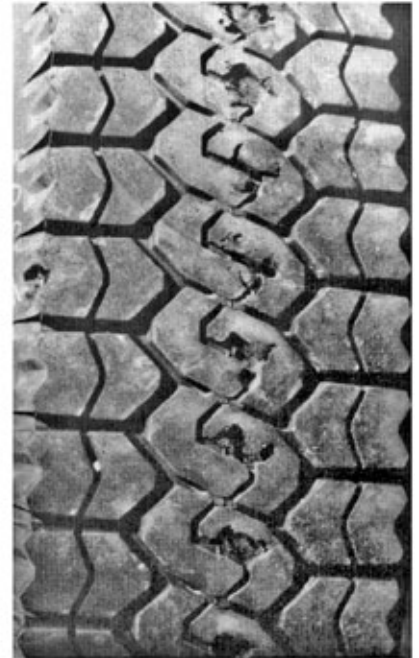
Example of Dyno Damage
